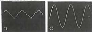
B—Shows output of low frequency driver when driven at a freq. of 22 Hz. Sound pressure reading, 90 dB. Note poor waveform. C—Output of venturi coupled duct, (under the same conditions as Fig. B.) Sound pressure reading 111.5 dB, (140 times more output than Fig. B.) Note sinusoidal (nondistorted) appearance.
